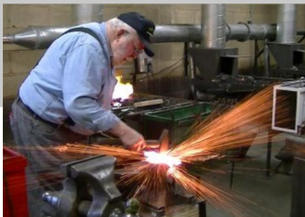
R. Rightmyer demonstrates forge welding a Damascus billet
